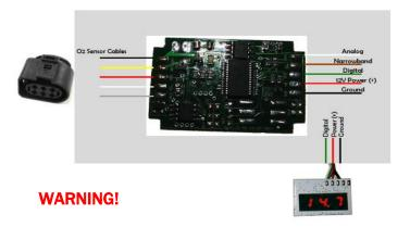
Oxygen sensor can get very hot when powered. Keep the oxygen sensor powered when the engine is running to prevent damage to the O2 sensor.
